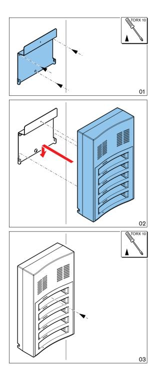
Figure 6.7: Installation to a wall
