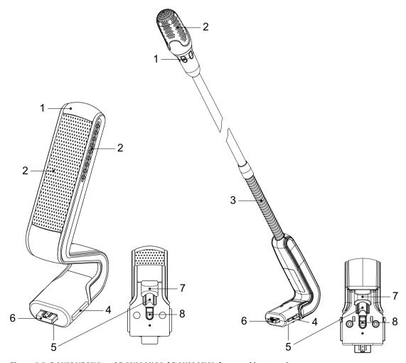
Figure 6.2: DCNM-HDMIC and DCNM-MICS / DCNM-MICL front and bottom view
