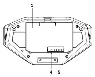
Figure 6.4: Wireless Device bottom view including Battery Pack
