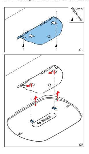
Figure 5.3: Mounting to a wall or ceiling
