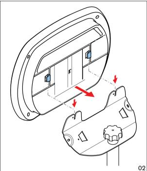
Figure 5.4: Mounting on a tripod floor stand
