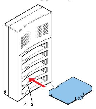
Figure 6.8: Placing of the Battery Pack
